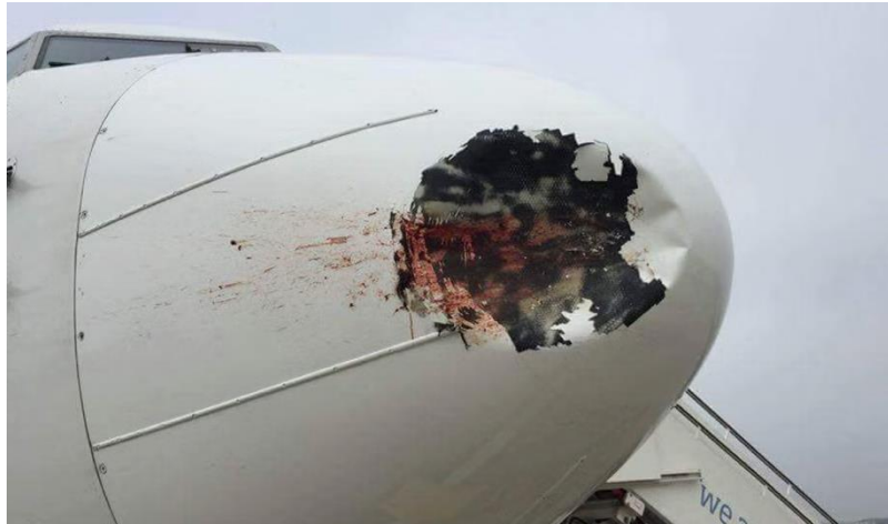
Figure 44. Image showing damage to a plane hit by a bird, made of low-density flesh and bone
