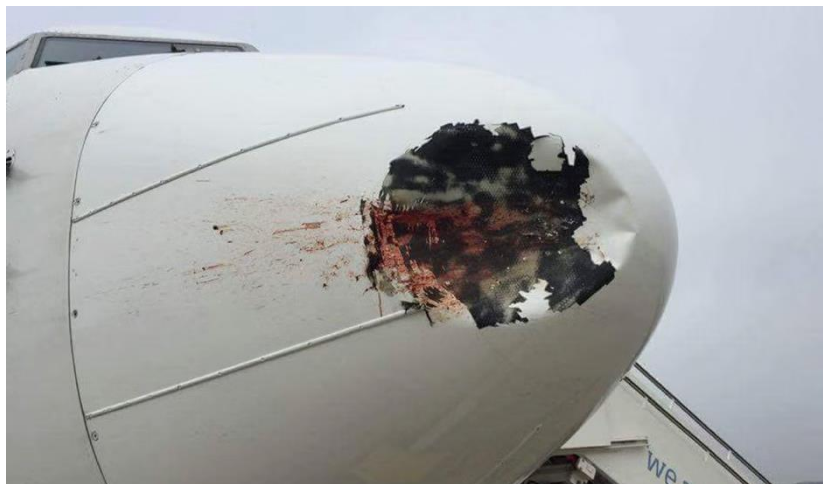
Figure 17. Image showing damage to a plane hit by a bird, made of low-density feathers, flesh and bone
