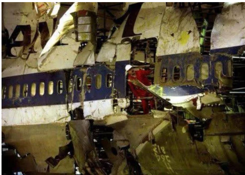
Figure 7. An image of the reconstructed Flight PA103, showing the part of the plane damaged when a bomb exploded in the luggage hold on 21 st December 1988
